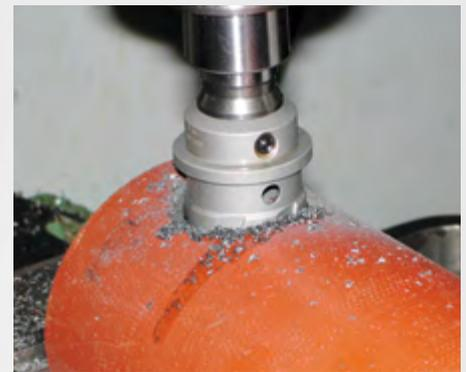
Bohren in Rohre
