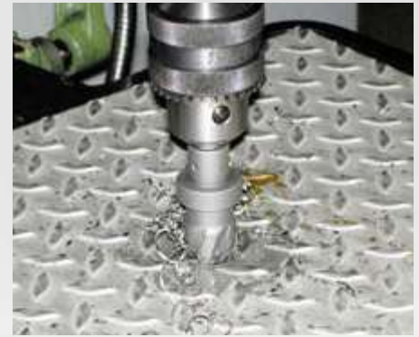
Bohren in Riffelblech
