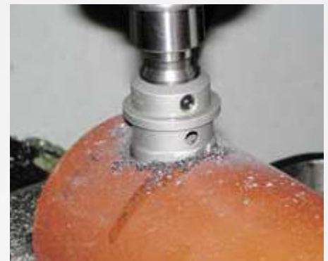
Bohren in Rohre
